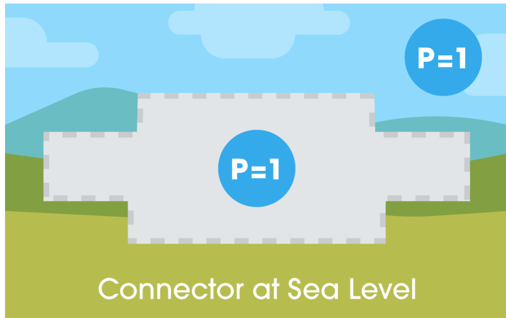
Figure 1: At sea level the pressure inside and outside the connector is 1 ATM
